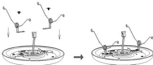
**STEP 4** According to the base can, the screw can be loosened to make 4-5-6in adjustment, and the 4-inch adjustment requires the entire spring tabs to rotate 180°, then fix it after rotation.
