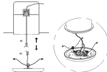
**STEP 7** Press the spring tabs of the fixture and fix it on the bracket of the recessed housing.
