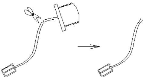
**STEP 4** Take out the AC line from the junction box, and connect it with the terminal of Line, N line and G line; L to L, N to N, G to G, Wiring connection, insert the wires into existing wiring connector of the fixture.
