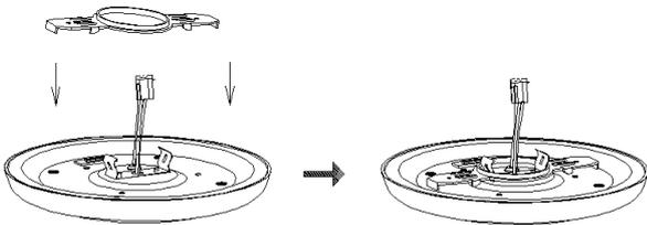
**STEP 3** Take out the spring tabs and screws, and install them on the fixture.
