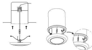
**STEP 8** Fix the whole fixture into the recessed housing to make sure it's firmly connected. After the installation is complete, check the wiring is safe before turn on the power.
