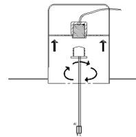
**STEP 6** Take out the fixture and connect the male and female quick connector.
