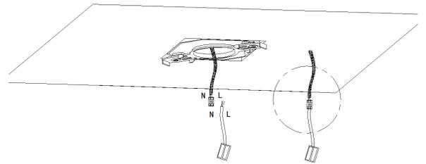
**STEP 5** Take out the fixture and connect with male and female fast connector. After ensuring it's firmly connected, tidy the wires and install them on the multifunctional bracket.
