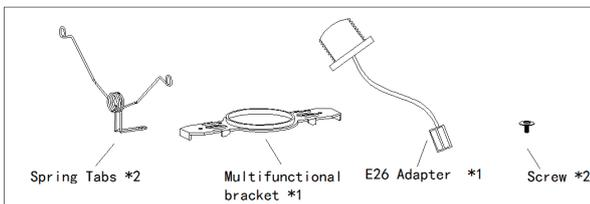
**STEP 2** Take out the fixture and install the multifunctional bracket on the back of it.
