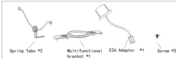
**STEP 2** Fix the multi-functional bracket to the junction box with screws according to the square shown in the figure.
